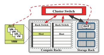
Figure 1: Data center architecture using networkbased storage. We show the typical data center design using racks of compute servers and storage servers. The data from the compute servers pass through the cluster switch to reach the storage rack. These rack-to-cluster links are *oversubscribed* leading to a bottleneck with higher server consolidation.
