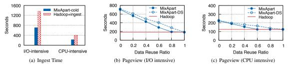
Figure 3: Analytics on a 100-core cluster with MixApart and Hadoop. We show *job durations* for a MapReduce job running on a Wikipedia dataset. The *CPU-intensive* experiment processes the *compressed* data; the *I/O-intensive* processes the *uncompressed* data. In (a) we run MixApart with a cold cache (MixApart-cold). In (b), (c) we run MixApart with a warm cache, with the data scheduler logic, and without (MixApart-DS).
